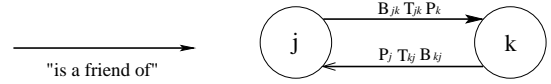
Fig. 1. Representation of balance and trust between peers in a p2p social network. The absolute balance between two nodes is the same in both directions, i.e., B_{jk} = -B_{kj} .
